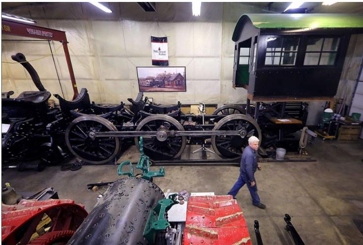
SPEC has hosted open houses each of the last three years on the same weekends as the Mad City Model Railroad Show & Sale but this year is skipping an open house to focus on completing the project. Plus, for the casual observer, the 40-foot-long chassis, with its three sets of 63-inch-diameter drive wheels, one set of which weighs 15,000 pounds, looks about the same as it did last year at this time.
